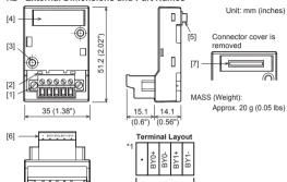
[1]Terminal block mounting screws [2]Output LED
